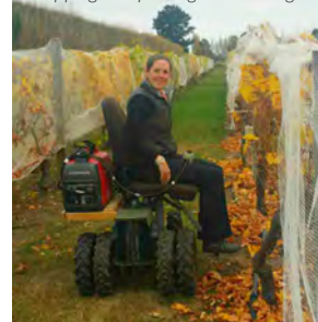
Student Mike Liao designed a machine for grape picking, leaf clipping and pruning while sitting.
